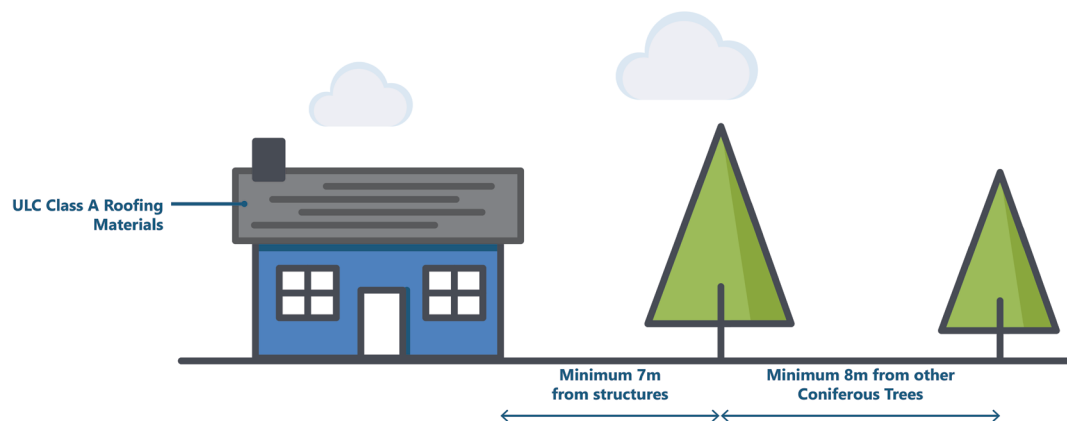
Figure 3.8.1(a) – FireSmart Roofing and Coniferous Tree Separation
